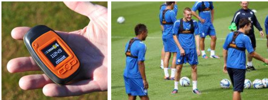
Figure 1. A typical sensor worn daily by football players to measure GPS and accelerations.
